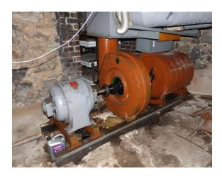
This picture shows the electric motor and the two blowing units. The bellows are the white bits in the background.
