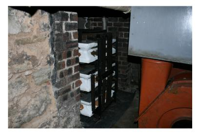
This picture shows the concussion bellows behind the blower. You can see the nice new white leather on the 3 bellows. Also, the frame that holds the bellows in place has been refurbished.
